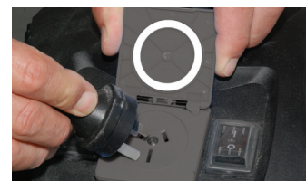
■ Sander power point and on/off switches
